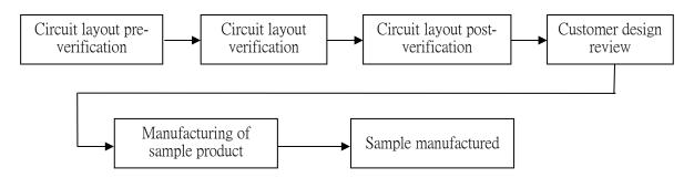
The second phase is to enter mass production of products verified by the customer. The production process of which is as follows:
